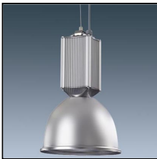
Type E High Bay With spun metal reflector (shown here) or with a prismatic reflector/refractor Lamps typically 250W or 400W and used at mounting heights typically 6m to 10m Used in industrial areas, retail sheds
